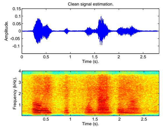
**Fig. 2.** Enhanced testing utterance in time and frequency domains when the proposed FPM noise estimation model is used with VTS feature enhancement.
